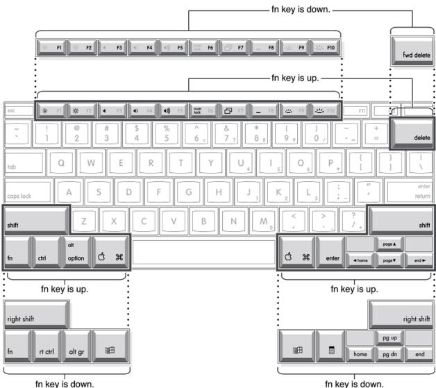
Figure 3-7 Alternate operations of function and control keys
